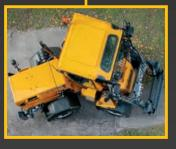
ARTICULATED STEERING Thanks to the articulated steering, the front and rear frames follow the trajectory of the work attachment. Working is more efficient and safer even in a confined, urban environment.
