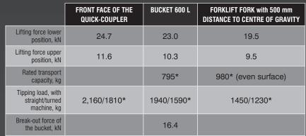
\* with rear-tilt, without counter-weight. According to the ISO 8313
