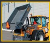
LOW REAR FRAME Thanks to the low rear frame, visibility to the rear is excellent. Work attachments may be hitched on top of the engine compartment.
