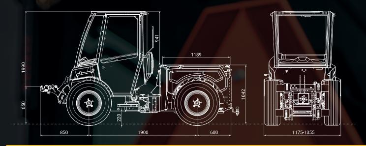
▶ Width 1175 / 1355 mm → Height 1990 mm → Length 3350 mm → Weight 2180 kg
