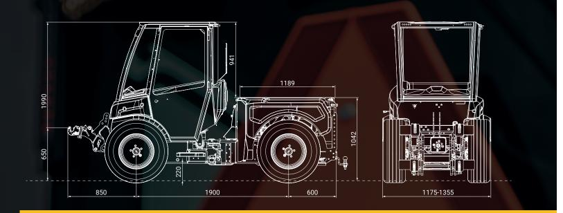
Width 1175 / 1355 mm > Height 1990 mm > Length 3350 mm > Weight 2180 kg
